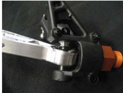
Lower arm installed on hub. Pivot ball long end down. (this is adjustable but may require mod) Roll center bushing on top.
