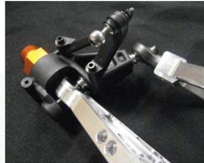
Assembled pic of both upper and lower arms on hub. Notice roll center bushing on upper arm attaching point.
